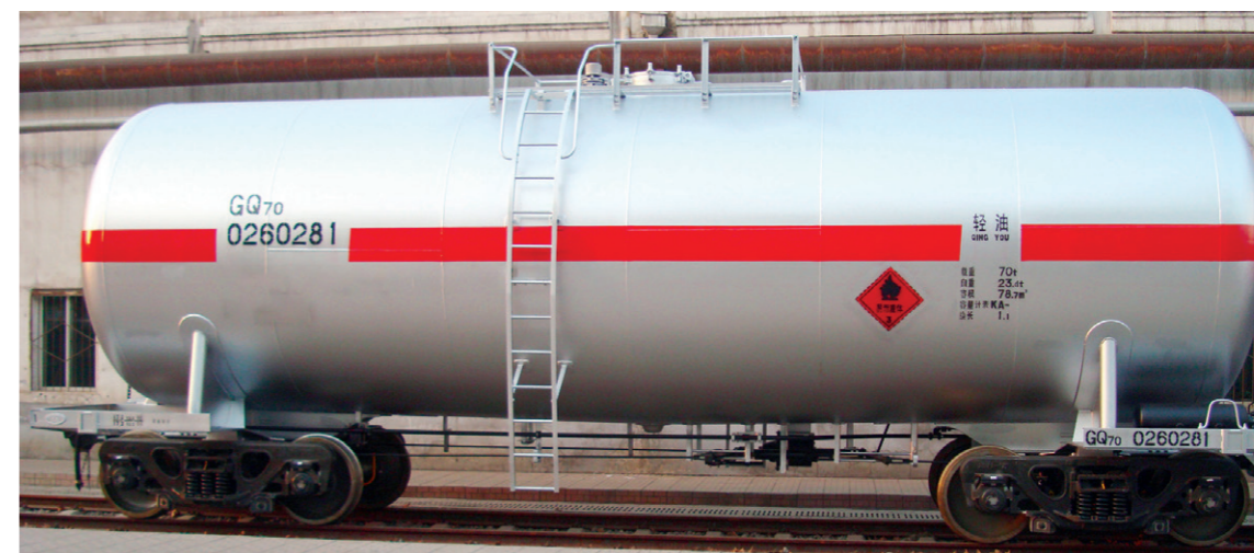
GQ70 型轻油罐车 GQ70 LIGHT OIL TANK WAGON
